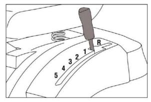
**A WARNING!** Only shift into reverse when the machine has stopped moving.
