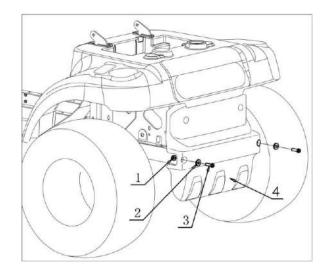
b.Insert the bushing (2) into the two holes where the bolts were just removed, align the towing plate (5),
