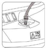
Connect a water hose to each of the pipe fittings one at a time and run water through each one for a few minutes, with the blades moving. When washing, the cutting deck should be lowered right down. Take off the grass-catcher, empty and rinse it, and then put it in a position where it can dry quickly.
