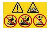
**Danger**: Risk of overturning on steep slopes Do not use the machine on slopes with a longitudinal gradient greater than 15 degrees (27%).
