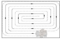
8. When you mow large areas, start by turning to the right so that the cut grass will discharge away from shrubs, fences, drive-ways, etc. After one or two rounds, mow in the opposite direction making left turns until finished
